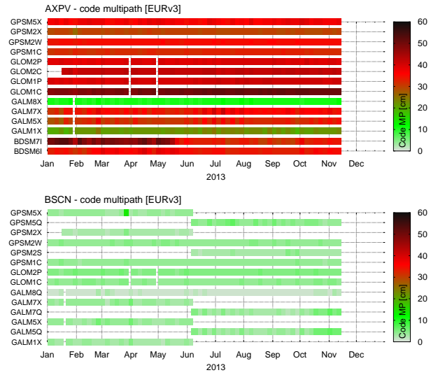
Fig. 2 Pseudorange multipath estimated for all GNSS signals observed at the EUREF station AXPV (top) and BSCN (bottom) during January–November, 2013
